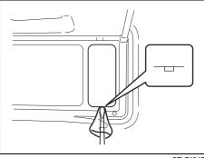
Pull down the lens by using a flat blade screwdriver covered with a soft cloth as shown. To install it, simply push it back in.
